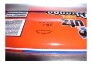
Thermal transfer overprinters feature a printhead and ribbon that make contact with a flexible substrate and create real-time images, including clean, high-resolution bar codes, text and graphics. For Utz, any product coding machine has to be robust enough to handle high line speeds while producing consistently readable codes. That was not the case with Utz's hot stampers, and also one of the reasons Epley first brought in thermal transfer printers.
